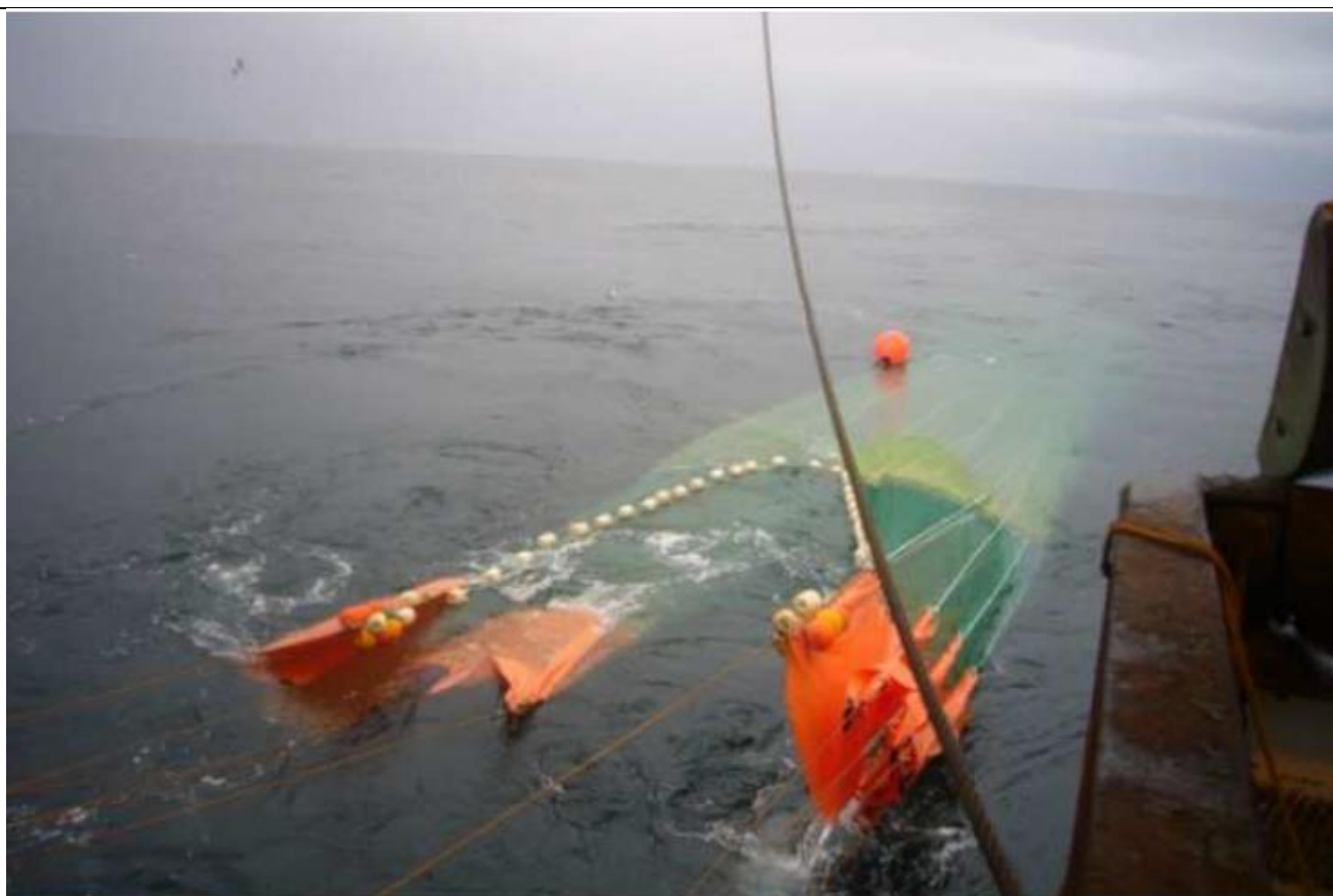
Figure 5: Full scale test of a commercial zooplankton trawl R30
