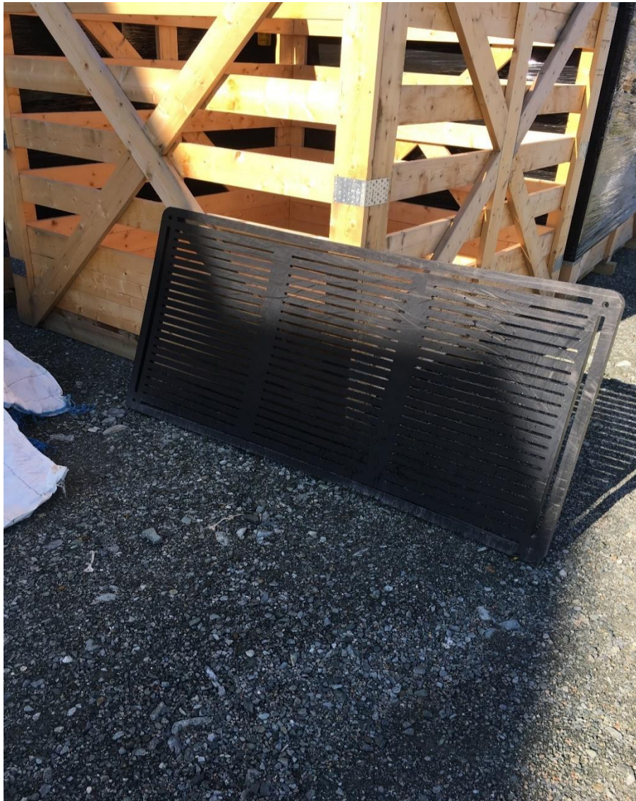
Figure 4: Calanus AS Bespoke Trawl sorting grid R23
