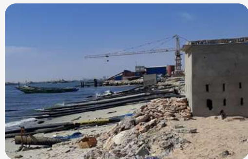
FIGURE 18: Pipes sucking fish from the boats into the factories and/or trucks in Mauritania
